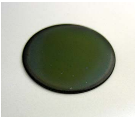
Figure 5a – Top view of a completed composite 1.25” wafer with 100- \mu m thick diamond
