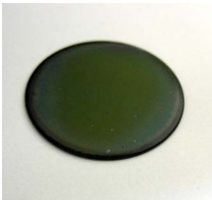
Figure 5a – Top view of a completed composite 1.25” wafer with 100- \mu m thick diamond
