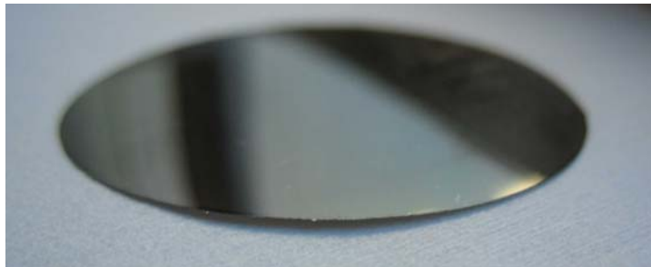
Figure 1. 2" diameter diamond wafer with 1 mm bow prior to mounting.
