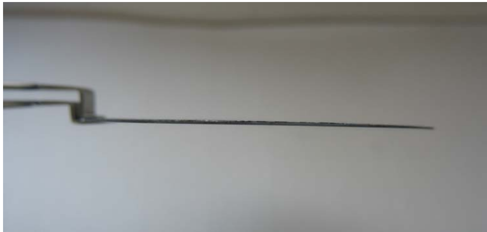
Figure 2. 2" diameter GaN-on-diamond wafer after mounting with semi-permanent bond (side view).
